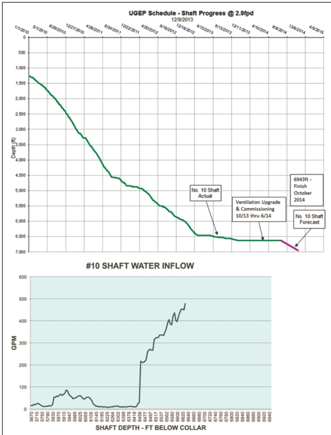
**Figure 2.** While drilling the No. 10 Shaft, the deepest single-lift shaft in the U.S., geothermal water (77°F) with a flow rate of 460 gallons per minute was encountered at a depth of 6458 feet, causing a two-year delay in drilling. By the time the shaft was completed at a depth of 6943 feet, the flow rate had increased to 1400 gallons per minute. Figure from E&MJ (2014).
