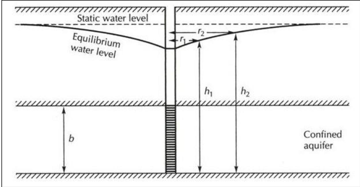
**Figure 3.** The Thiem Equation is used to calculate the steady-state discharge of groundwater into a well, based on the transmissivity of the aquifer and the heads at two distances from the pumping well. If  $r_1$  is equal to the well radius, then  $h_1$  is the water level in the well. At a sufficient distance from the well (called the radius of influence of the well), the head retains its equilibrium level and is undisturbed by the presence of the well. Figure from Fetter (2001).
