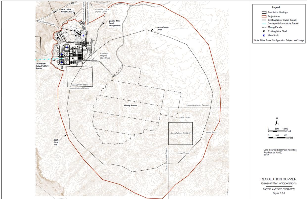
**Figure 4.** The underground portion of the Resolution Copper Mine would be beneath the East Plant Site. For estimation of the flow rate of geothermal water, the underground operation was approximated as a circle with a radius of 1400 meters. Figure from Resolution Copper Mining (2014b).
