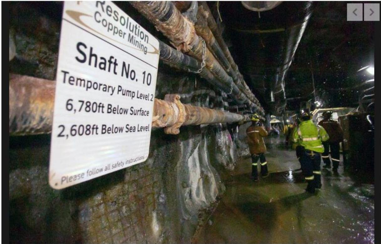
**Figure 5.** Based on the photo, the pipe diameter for mine dewatering was assumed to be six inches. Moreover, since the pipe in the photo is horizontal, the assumption that mine dewatering is accomplished through a single vertical pipe is a best-case scenario. The photo caption clarifies that the photo shows “pipes that move water...to pumps that send it to a water treatment facility on the surface” (Bregel, 2016). Photo from Bregel (2016).
